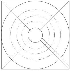
Mark the board on both sides with corner-to-corner lines to find the centre. Add a second line 10 mm away from one arm of the X and the same side of the same arm on the other side of the board. These lines will assist with alignment when gluing the parts later.
