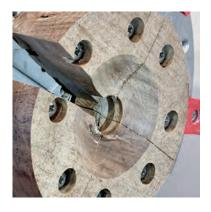
With the soft-grip jaws closed cut the centre to be slightly smaller than the half-spoon blank. Ensure that the top edge of the cut is a slight overhang and the bottom of the cur will support the bottom of the half-spoon blank.
