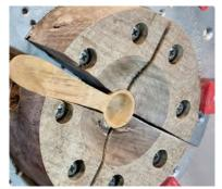
Grip a half-spoon blank in the jaws and hollow it out. Sand this cut area.
