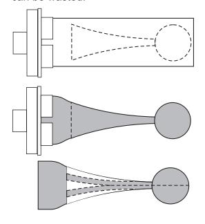
Mount a 40 mm x 40 mm x 130 mm long blank by one square end in a scroll chuck.
