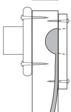
Put one spoon blank in the block on the lathe. Screw the mdf back onto the block. Through the hole in the mdf hollow the spoon. Sand the inside of the spoon.
