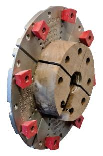
Or, for longer life of the soft jaws, drill holes and fit bolts, with the heads deep in the wood, to hold the wood segments to the Cole jaws.
