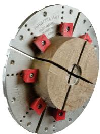
Use a bowl blank of 200 to 250mm diameter, 50mm thick and of firm wood. Turn it round on the lathe and then cut it to quarters. Secure this in a Cole chuck with the quarters exactly on the quarters of the chuck. From the back of the chuck put at least two screws into each quarter of the wood.
