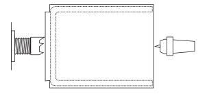
For the body of the pot start with a block of wood that is 100 mm square and 140 mm long. The grain should be along the long axis. Mount this between centres and turn it round. Cut an 81 mm spigot for holding it in a 100 mm chuck at the end that is to be the bottom.
