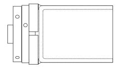
Mount the wood in a 100mm chuck. Turn the outside down to 87 mm diameter. Hollow the inside to leave about a 6 mm wall and bottom thickness. Sand and finish as much as possible of all surfaces. If you are planning a band of decoration on the pot you can mark the area to be decorated at this time.
