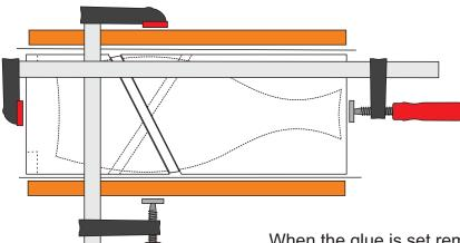
Clamp the parts together. Do this on a flat, clean table with paper under the block. Put paper along each side of the block and then a clamping block on each side. Finally clamp the parts both laterally and longitudinally. Ensure that all parts are correctly aligned.
