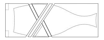
You will note that your planned second cut is no longer true due to the first laminate being thicker than the first cut. Re-design this second cut so that the laminates will cross at the centre of the wood. Cut the wood and make the faces perfectly flat. This cut may be the thickness of your saw blade or you may make exactly the thickness of the laminate. Cut the laminate to fit within the width of the block. Apply glue to both faces of the block and both faces of the laminate.
