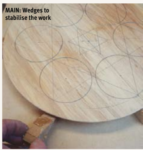
MAIN: Wedges to stabilise the work
