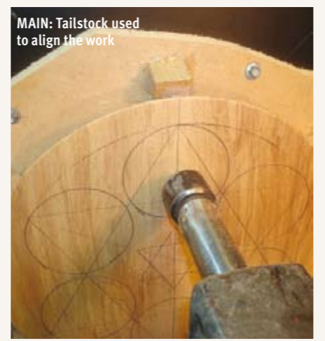
MAIN: Tailstock used to align the work
