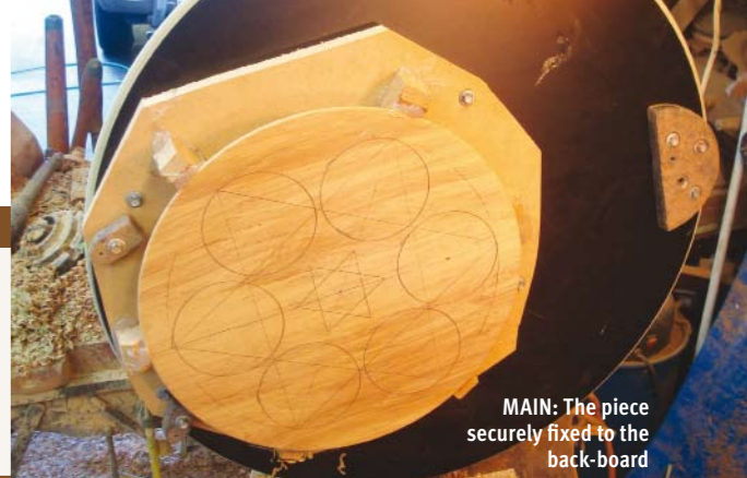
MAIN: The piece securely fixed to the back-board
