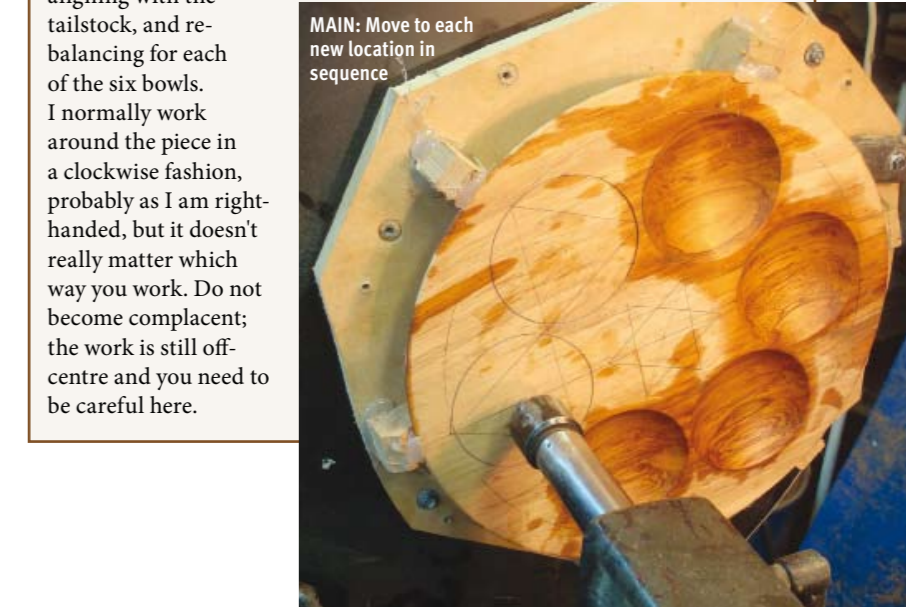
MAIN: Using the depth guide to check the work
