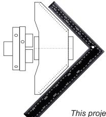
Cut the block to the shape shown. There needs to be a 90° angle between the two sides. Use a carpenters square placed exactly on the cut lines to achieve this. Sand this surface to a finished quality.
