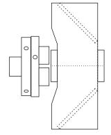
Turn the wood over and mount it in a chuck. Turn it round and 191 mm diameter. Turn a chuck-mounting spigot on the exposed side.
