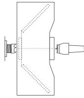
Mount the wood on the lathe. Use a very wide faceplate or mount between centres. Other mounting methods may split the paper joints or damage the finished work. Cut a chuck-mounting spigot on the side that will be the wider side of the turning.
