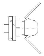
Turn the wood over and cut out the centre of the bowl. Tape the extremities of the bowl to stop premature parting of the segments. Maintain even thickness as you work down to finally part the four segments off the bowl. Hand sand the inside of these.
