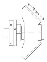
Cut the outer corner of the bowl shape away. This cut should be at right angles to the sanded surface of the bowl and allow for the cutting of a 3 to 5 mm thick bowl wall. At a point 80 mm from that outer edge cut at right angles into the bowl deep enough to allow for the cutting of a 3 to 5 mm thick bowl wall.
