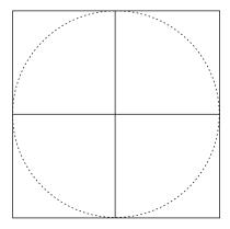
Start with two blocks of wood that are 200 square and 80 mm thick. Cut each block into quarters and then dress the inner faces and rejoin the blocks with paper joints. You may cut and rejoin the blocks on diagonal lines which will give a better grain match in the finished work but may result in more splitting of the edges. When the glue is dry, cut these blocks to round on a bandsaw.
