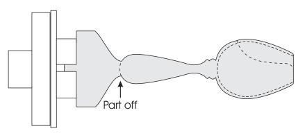
Work the very bottom of the outside of the scoop and the handle down to shape while leaving an adequate attachment to the chuck. Sand and finish the outside of the scoop and handle.
