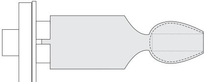
Drill the centre out of the scoop and then continue to hollow the inside.
