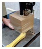
1. Cut the wood for the project to size. Be sure to have enough for drive and tail centres or a chuck spigot. You may make a slight increase in width to allow for the width of the next bandsaw cut.
