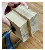
6. Put the blocks together with the paper layer between. Rotate one block now if it needs to be rotated back again later to maintain a grain match. Clamp lightly.
