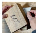
7. Rotate the block to match the angle template made earlier. Clamp lightly.
