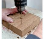
2. Measure the diameter of a thin dowel. Bamboo skewer is suggested. Drill a 5 mm deep hole of that size in the centre of each face.
