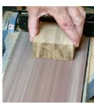
4. Sand the two faces from the last bandsaw cut to ensure that the wood is flat and free from saw marks.
