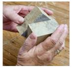
5. Rub the blocks together to spread a thin layer of glue on both blocks.
