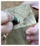
2. Mark one face of the block clearly with a pencil line or two. This ensures that you will know the original orientation of the parts of the wood after the next bandsaw cut.
