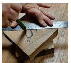
8. When the glue has set, mark the centre of one side of the glued blocks. Draw these lines well towards the corners of the block.
