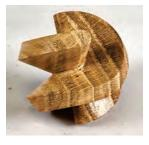
10. Sand the remaining paper off while keeping the surfaces perfectly flat. Glue the parts together. Rotating one if needed to match the grain.
