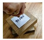
9. Cut a paper or card template to the size of the planned block. Place it centrally on the marked lines on the wood. Draw lines at the edges of this template.
