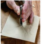
3. Prepare paper for the joint. Cut it slightly smaller than the wood face. Mark the centre and punch or cut a hole at that point.
