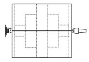
Turn the wood to be round and 60 mm diameter. Measure and mark a line at the exact centre of the length of the wood. Then mark lines at 6, 18 and 30 mm each side of the centre line. On both ends of the wood mark lines that are 12 and 24 mm in from the 60 mm diameter of the wood.
