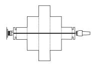
Re-draw the two lines that were 30 mm from the centre line onto the newly cut surface of the wood. Keep all cuts straight and clean. Start a parting off cut on the outer side of each of these 30 mm marks. Sand all surfaces.
