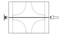
Turn the wood to be round and 60 mm diameter. Measure and mark a line at the exact centre of the length of the wood. Then mark lines at 5 mm and 30 mm each side of the centre line.
