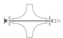
Cut a curve that extends from each of the lines you drew 5 mm to left and right of centre to the lines you made at 30 mm from centre on the 10 mm diameter wood. The length and curve of this should be the same on both ends of the wood. Start a parting cut immediately outside the 30 mm marks on the 10 mm diameter wood. Sand all this cut surface. Part the work off and hand finish the ends.
