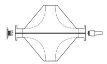
Cut away the corners of the wood and turn both ends of the wood down to 10 mm diameter.
