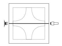
Start with a block that is two halves of a 75 mm cube cut and rejoined with a paper or double-sided tape joint at the centre. Mount this accurately between centres with the joint perfectly on centre and in line with the lathe drive.
