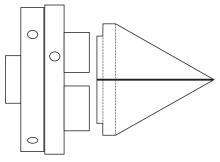
Turn the wood to a cone shape between the 52 mm mark and the pencil dot on the end. Sand and finish this surface.
