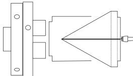
You now need to turn the wood around to finish the other end. Make a jam chuck and use Tape or hot melt glue to hold the wood while it is turned. Bring up the tailstock for added security. Turn the tailstock side to be perfectly flat. Sand this side
