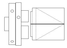
Mount the work in a chuck. Turn it to exactly 60 mm diameter. Dress the tailstock end of the wood to be flat and put a pencil mark at the centre. Mark a line around the wood 52 mm from the tailstock end.
