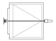
Start with a block that is two halves of a 65 mm cube cut and rejoined with a paper or double-sided tape joint at the centre. Mount this accurately between centres with the paper joint perfectly on centre and in line with the lathe drive. Round it off and make a spigot for a 50 mm chuck on one end.
