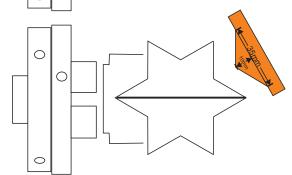
Cut a straight face between the 52.5 mm line and the centre of the end.
