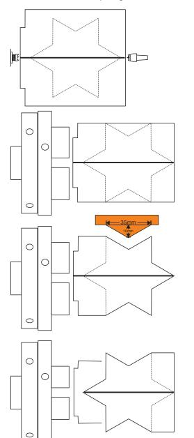
Start with a block that is two halves of an 80 mm cube cut and rejoined with a paper or double-sided tape joint at the centre. Mount this accurately between centres with the joint perfectly on centre and in line with the lathe drive. Turn the wood to be round and cut a spigot for mounting the wood in a 50 mm chuck on one end.
