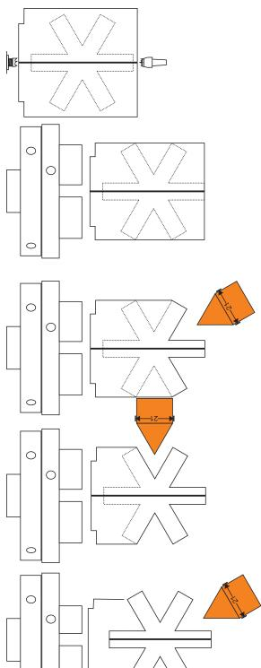
Start with a block that is two halves of a 70 mm cube cut and rejoined with a paper or double-sided tape joint at the centre. Mount this accurately between centres with the joint perfectly on centre and in line with the lathe drive. Turn the wood to be round and cut a spigot for mounting the wood in a 50 mm chuck on one end.
