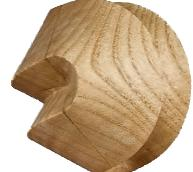
Remove the wood from the lathe. Split the joint and ensure the two faces of the wood are clean and smooth. Rotate one of the two parts through 90 degrees and glue the wood together. Sand and finish.
