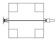
Turn the wood to be round and 60 mm diameter. Measure and mark a line at the exact centre of the length of the wood. Then mark lines at 15 and 30 mm each side of the centre line. From outside of the 30 mm lines cut both ends of the wood perfectly flat, but leaving the wood the drive spur and live tail are pressing on. On both ends of the wood mark a 30 mm diameter line.
