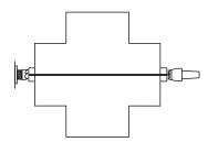
Cut away the wood as a square between the 15 mm marks and the 30 mm diameter lines on each end of the wood. Keep all cuts straight and clean. Sand all surfaces.
