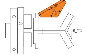
Start with a block that is two halves of a 70 mm cube cut and rejoined with a paper or double-sided tape joint at the centre. The grain direction of both halves should be along the bed of the lathe. Mount this accurately between centres with the joint perfectly on centre and in line with the lathe drive. Turn the wood to be round and cut a spigot for mounting the wood in a 50 mm chuck on one end.
