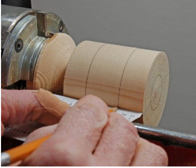
Fig02: Using the larger scale to measure away from edge of the cylinder.
