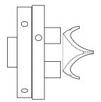
Cut the wood to the shape shown. The outer edges are turned down to the thickness mark. The centre remains at the height cut before the hole was drilled. Ensure that the centre piece around the drilled hole is just under 4 mm diameter so that it fits into the 4 mm hole in the neighbouring segment.
