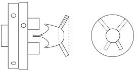
Turn the wood over and mount it in a smaller chuck. Turn the wood round and down to a diameter that will give you eye stalk lengths of your choice. Then cut away the centre of the head and behind the eye stalk to leave a disc of wood. You can now carve that disc of wood to be the eye stalks and antennae.
