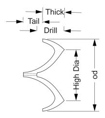
The 17 body parts are all the same style but of differing sizes as listed in the table below. Start by cutting 17 blocks that are 50 x 50 x 35 mm. If possible the grain direction should be along the 35 mm axis.
