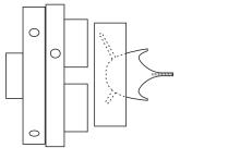
Turn the narrowed down part of the wood as shown. Ensure that the central extension is just under 4 mm diameter at the tip to fit into the adjoining body part. Note the sloping start to the head shape. It is necessary to cut this part now so that a small chuck can hold the head. Sand this area.
