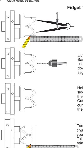
If needed, true the face of the wood. Mark on that face the High Diameter (H Dia in the table). Mark on the side of the wood the Thickness (Thick in the table) of the segment you are turning.
