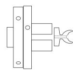
Hollow the end of the wood down to almost the bottom of the 4 mm drilled hole. Curve the outside of the block as shown. Sand this area. Part it off.
