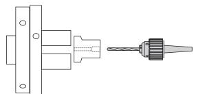
Cut a block of wood 20 mm on all sides. Mount this in a small chuck. Turn it down to 15 mm diameter. Drill a 4 mm 6 mm into the wood. Then a 1.5 mm hole completely through the wood.
