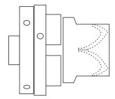
Start with one of the 50 x 50 x 35 mm blocks mounted in a chuck. Ensure that at least 25 mm of the wood is protruding from the chuck jaws. You may need to put a packer behind the wood. Turn the wood to the od, as shown in the table, of the segment you are turning.
