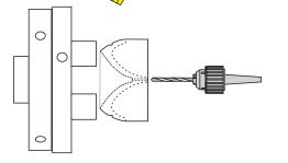
Cut the wood down to the Tail Length mark. Drill a central hole completely through the wood, 1.5 mm diameter is recommended, for the string.
