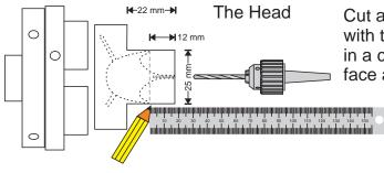
Cut a block of wood that is 50 x 50 x 40 mm with the grain along the 40 mm side. Mount it in a chuck and make it round. Dress the outer face and drill a 1.5 mm hole 15 mm into the
