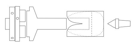
Mount the wood on the mandrel and bring up the tailstock to hold it in place. Turn the wood to round. Run a pencil mark round the wood at about one third of its length from the tailstock end. This should remain as the broadest part of the flower.
