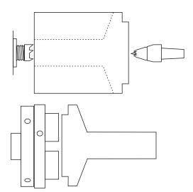
Mount this wood between centres. Turn it to round and then turn a spigot for a 50mm chuck on one end.
