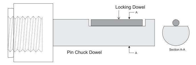
A pin chuck with a 25mm shaft, a flat cut 6mm into the shaft and 6mm locking dowel. This is made or mounted on a plate which can be held in a four jaw woodturning chuck or be threaded to fit the lathe drive..
