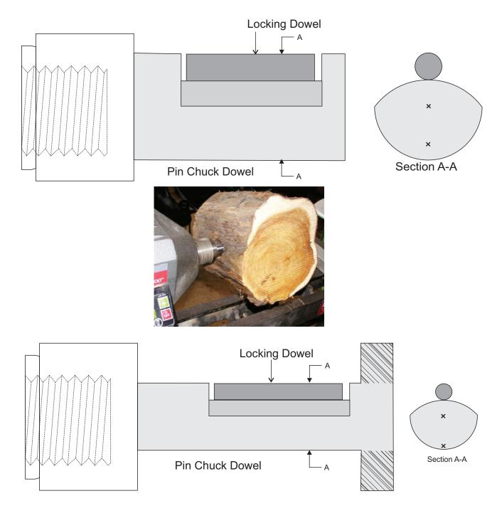
To get a similar curved seat for the dowel on smaller pin chuck. Turn the main shaft to size but leave the end full size. Remount the wood between centres that are about 12mm offcentre. Turn the curved seat for the dowel. Remount the work between its true centres and remove the excess wood at the end.
