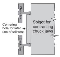
The traditional recommendation is that the spigot is cut at a slight angle. This angle must be very slight (for Nova jaws) as the protrusion from the jaw that grips the wood extends just 0.5 mm from the jaw surface.
