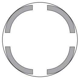
If the dovetail is cut to 70mm then the chuck jaws will press on the wood at only four points.
