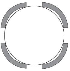
If the spigot/tenon is cut to 65mm then the chuck jaws will grip the wood at only 8 points.
