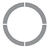
Teknatool 50mm chuck jaws as made. A perfect circle with an inside diameter of 44.5mm and outside diameter of 53.5mm.
