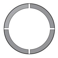
If the dovetail is cut to 54mm then the jaws will press evenly on the wood all around the dovetail.
