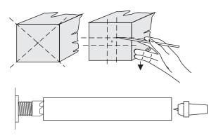
Mark the ends of the wood to locate the centre. Secure the wood firmly between the spur drive in the head stock and tail stock centre. Make sure the spur drive is driven well into the wood and the tailstock is secured.
