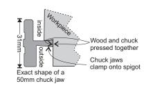
A more accurate cut, particularly for hard woods, is to make a spigot with no angle and then to cut a sharper angle close to the base of the wood. As the chuck is tightened the jaws are drawn firmly to the base of the work.
