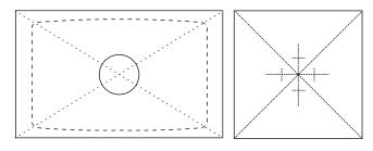
Start with a block of heavy wood 130mm long and 80mm thick both ways. The grain should lie along the long axis. Drill a 25mm hole through the centre, across the lie of the grain.
