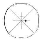
Remount the block between centres with both head and tailstock at the offset markers to the same side of centre. Turn that face just up to the longitudinal pencil marks. Repeat for each face. Sand the faces longitudinally to preserve
