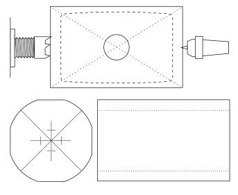
Mount this block between centres. You do not need to round it off completely. Turning the offsets later will take away about one quarter of the width, ie one eighth either side of the centre line of the original flat face.
