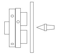
Make two disks for the ends of the drum that rides on the back of the snail. Use thin hardboard or plywood. Hold it firmly against a chuck or a block of wood held in a chuck. Hold it in place with a pointed live centre. This pont mark will be used as the mark for attaching the disk to the drum. Turn each disk to 85mm diameter. Sand them and paint them the colours of your choice.
