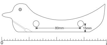
The body of the toy is 175mm long and cut from 20mm thick wood. Drill 11mm holes for the wheel axles and an angled hole for the string. For tidiness make the lower end of the string hole larger to accommodate a knot at the end of the string. Sand all surfaces and apply a finish or colour of your choice. Paint on or glue on eyes.
