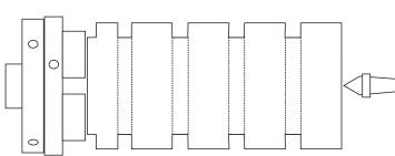
Part off the first 20mm thick wheel. Hand sand the back of the wheel. Sand the end of the wood on the lathe. Repeat this process until four wheels are completed. Drill a 10mm hole in each wheel 2mm offcentre. Cut lengths of 10mm dowel and fit the wheels to the body. Place the offsets of each pair of wheel opposite to maximise the waddle of the duck.
