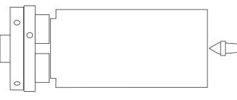
For the wheels start with wood that is 70 x 70 x 120mm long. Mount this in a chuck and turn it to 60mm diameter. Sand this surface and the end of the wood. Do not drill a central but bring up a pointed live centre to mark the centre of each wheel.
