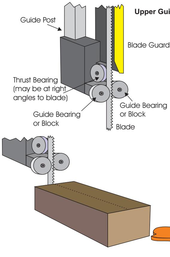
Before use, check the blade sharpness and tension. Check that the blade guides and thrust bearing are in place and nearly touching the blade.
