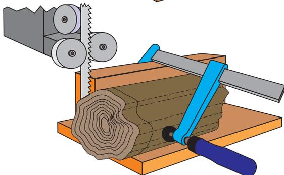
To cross-cut round or irregular wood clamp the wood securely to a wood fence which is large enough and strong enough to stop the rolling action that the bandsaw will impart on the wood. Keep the edge of the supporting wood as close as possible to the bandsaw blade.
