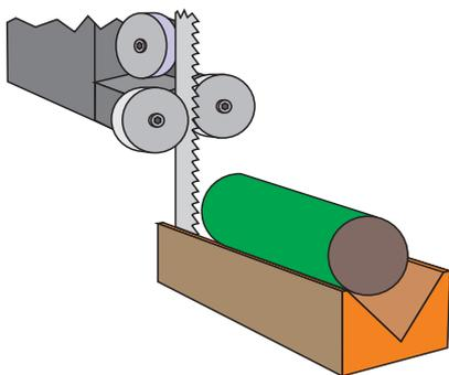
To cut round or uneven wood lengthwise put the wood in a Vee cut trough so that it sits firmly without wobble or wiggle. The bandsaw cut will also cut through the supporting wood so ensure that it is longer than the project wood or make several cuts moving the wood within the trough for each cut.
