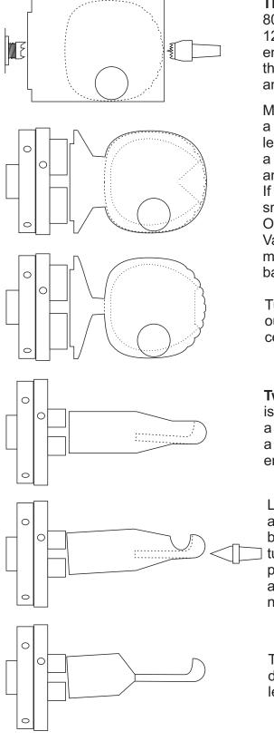
**The Shell**. Start with a block of wood that is 80mm long and 60mm square. On a centre that is 12mm from the edge and 35mm from the tailstock end drill a 20mm diameter hole through it. Mount the wood between centres, turn it almost round and cut a spigot on the headstock end.
