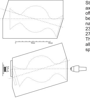
Start with a block 180 x 110 x 80. Mark the vertical axis on centre at both ends. Cut an angled piece off the block at both ends, and opposite sides, between the centre point and 17mm down the narrower side. Mark the angled centre on this cut 23mm from the vertical centre on the top end and 27mm from the vertical centre on the foot end. The greater distance off-centre at the foot end allows for the greater length needed to include the spigots.
