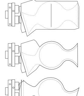
Mount the wood in a chuck using the spigot on the angled centre. Turn the area that is to be the body and upper part of the vase down to a diameter of 77mm. After making allowance for wood to be removed at the top end and between the spigot and foot, put a pencil line around the body of the vase at the mid-length point.
