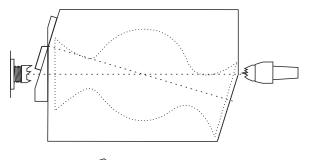
Remark the vertical centre on the bottom end of the wood. Remount the wood on the vertical centres and cut a 46mm diameter spigot at the foot end. The length of this spigot will be between 8 and 10mm. Ensure that it is not too long to fit the chuck.
