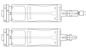
Mount the wood in a chuck and bring the tailstock up. Turn the end 53mm down to 15mm dia. Mark the wood with 2mm to be taken off the end to remove the tailstock marks and 20mm for the boots. Drill a hole into the uppermost part of each boot to glue the leg string into later.
