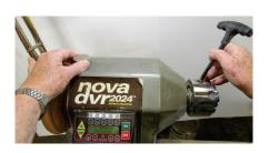
To safely mount the wood. Rotate the chuck so that a keyhole is uppermost. Lock the spindle and keep it locked while mounting the wood.
