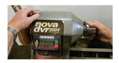
When the user has a dig-in the chuck may become jammed on the lathe spindle due to the chuck not being seated snugly against the headstock bearing. Follow these instructions to prevent this happening. Lock the lathe spindle.
