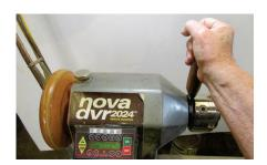
Use the spanner to firmly tighten the chuck on the spindle
