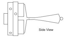
Cut the upper end of the pendant thinner. The narrow end needs to be the shaped to fit a pendant clip or a hole drilled for a ring. Sand and finish all surfaces. It may be easier to add embellishment while it is held in the chuck. Part off.
