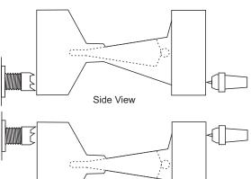
Remount the wood by one off-set. Turn that side down to exactly the pencil line at the wide end, but stay a couple of millimetres away from the pencil line towards the narrow end of the part you are cutting. This edge can be sanded on both sides to meet later.
