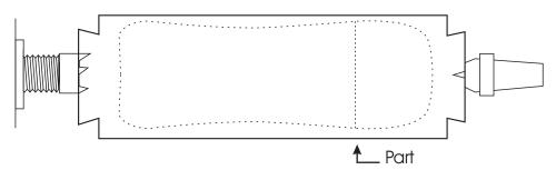
Round off and cut a spigot on both ends. Part off where the top/bottom separation is to be. Allow for a generous overlap when the two parts are brought back together.
