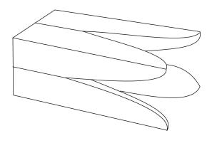
Break the paper joints apart and reglue the blocks with permanent glue in the form shown.
