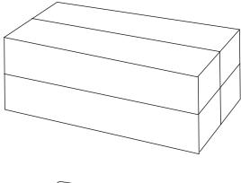
Dress four lengths of wood so that they have a square cross section. Glue them together with paper joints.
