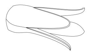
Put this glued block back on the lathe and turn the outside of the flower petals, including around the base. Sand and finish.
