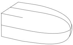
Mount this block on the lathe so that you can turn it to the shape shown. Sand and finish the surfaces that have been turned.
