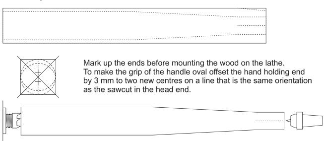
Mount the wood between centers on the center point of each end. Turn it round and down to about 32 mm diameter. Turn the hammer head end to a good fit in the previously drilled hole in the head. Slope the handle from about the centre point to this diameter. You may fit the handle and head together and use it like this. OR continue as below to make an oval handle
