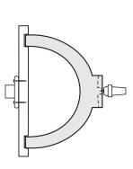
Turned to fit wooden chuck, or jam chuck. Best used with the tailstock in place or tape or hotmelt glue as added as security. If the jam chuck fit is good, the tailstock can be removed for cutting the last little spigot and sanding.
