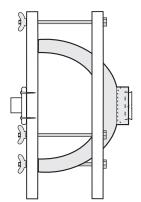
A compression chuck is a faceplate on the lathe spindle. A board of similar size is cut to a donut and fitted over the bowl, clear of the bowl bottom, and held in place with bolts. The bowl bottom can then be cut away and finished.
