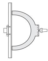
The tailstock can be used to hold the bowl against a large padded faceplate. The last little spigot between the tailstock and the bowl foot is cut off after the bowl is taken off the lathe.
