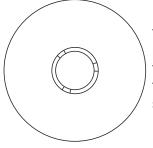
Use the lathe index or a template to mark the circular foot into equal portions, usually thirds, and decide the width of each foot. Cut away the unwanted wood and sand the surface down to a perfect curve.
