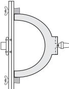
A Longworth Chuck or Cole Jaws grip the outside (or inside) of the bowl rim. Initially this is best used with the tailstock in place. But the tailstock can be removed for cutting the last little spigot and sanding.
