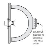
A vacuum chuck is used with a vacuum cleaner or vacuum pump sucking through the centre of the faceplate. This pulls the bowl onto a closed cell foam layer on the faceplate. Initial positioning of the bowl
