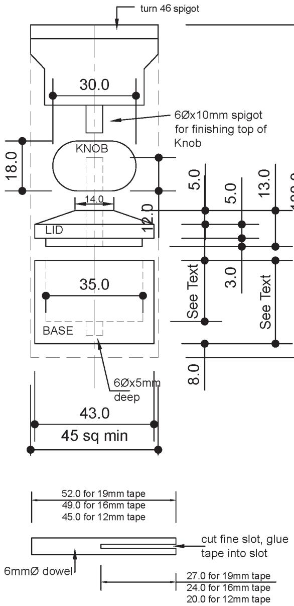
Start with a block at least 45mm square x 120mm long. Mount it between centres and turn a 46mm spigot on the headstock end.
