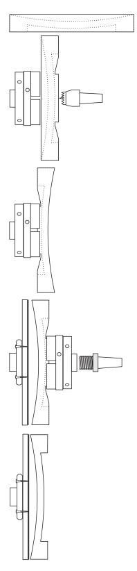
Start with wood that is 180mm square and 25mm thick. It should be dressed on all four of the narrow sides and the side that is to be the bottom. Mark the centre on the bottom.
