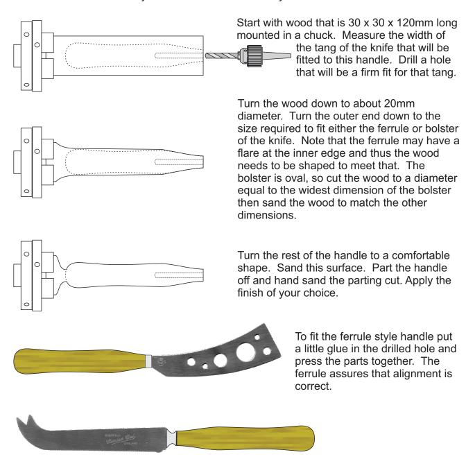
For the bolster style fitting care needs to be taken with alignment of the bolster. Put a little glue in the drilled hole and around the lip of the hole. Bring the parts together and then align the bolster and hold it in place until the glue is set.
