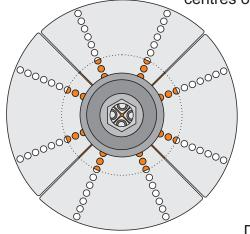
Place the Cole jaws face-down on the block of wood. Look down through the chuck to find and position the centre-point of the wood as now marked by the drive centre on the lathe. Then mark on the wood the centre of each screw hole that will be used.
