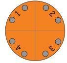
When all holes are drilled mark where the block is to be cut to quarters. Write numbers on the quarters to assist with repeated re-assembly of the ball chuck. Cut the block to quarters.
