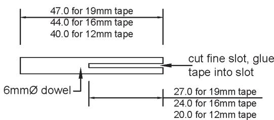
**Assembly.** Glue the dowel into the knob. Slide the lid up the dowel to the knob. Bend the metal inner end of the tape so that it will go through and then wrap around the dowel. Then glue it to the dowel. Pass the tape through the slot in the side of the body and seat the lower end of the dowel into the hole in the base. Seat the lid onto the body with a little glue to keep it there. Turn the knob to wind the tape into the body.
