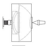
Mount the round block on a broad faceplate or between centres. Turn only a spigot for the planned box bottom. The size of this will be determined by your overall box size but a 47mm spigot for a 50mm chuck is recommended. Mark the centre of the spigot.
