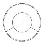
Mark up the top of the block. Use a compass with a pencil to draw, based on the centre point of the block, a circle towards the edge of the block. Keep that compass setting and step around the line you drew to mark it into six equal segments. Continue three of those marks at the one-thirds points boldly for about 10mm down the side of the block. From the other three marks draw a straight line towards the centre of the face. Reset the compass to the radius of the block.
