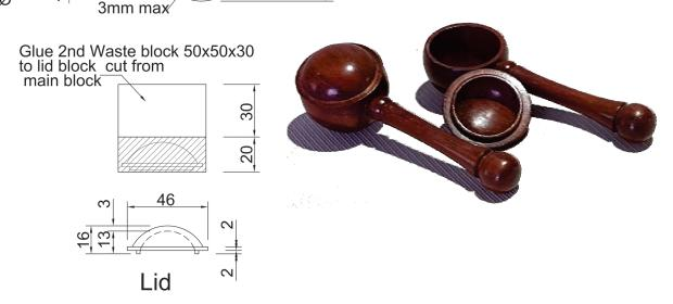
Make a jam chuck that will hold the spoon with the bandsawn face parallel to the face of the chuck. Turn off the last of the waste block and hollow the spoon to 3mm thick. Sand and finish. Remove the spoon from the jam chuck.
