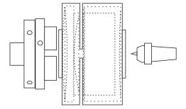
Mount the chosen wood between centres. Round it off and make a chuck bite spigot on both top and bottom. Mount this in a chuck by the side planned to be the top of the box.
