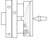
Mark the centre of the flat side of the jewellery wood (which is still square at this stage). Place the tailstock centre at this point and move the tail and wood up to the chuck.
