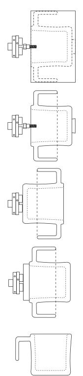
Mount the wood on screw chuck, or make a spigot and mount it in a chuck.
