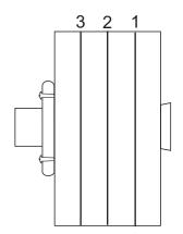
Mount the blank on a faceplate or screw chuck. Round it off and cut a spigot (chuck bight).
