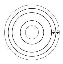
On the flat you have just cut mark a line at half the distance from the second circle to the edge of the round.
