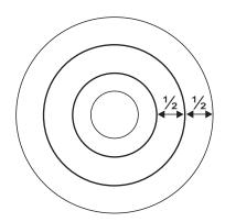
On the flat you have just cut mark a line at half the distance from the first circle to the edge of the round. Cut straight from that line to the left hand mark (line No 3) on the rounded side.
