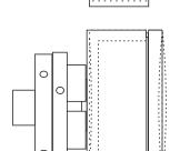
Fit the box top onto the box bottom. Cut the sides of the box down to the exact width of the top.
