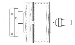
Mount the chosen wood between centres. Round it off and make a chuck bite spigot on both top and bottom. Mount this in a chuck by the side planned to be the top of the box.
