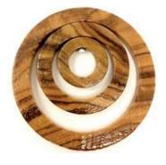
Rings cut for inlays need to be made with a grain orientation that matches the form they will be fitted into. The cuts need to be smooth but sanding should not be necessary.
