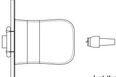
Turn the pot around and remount it on a vacuum chuck, Cole jaws, jam chuck, or pressed to a rubberised faceplate. Cut off the spigot to leave a slightly concave surface.
