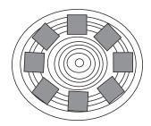
Cut rings 150mm thick from a fresh-felled log or large branch. Mark out one side of that blank and then cut on a bandsaw 100 x 100mm blocks. To reduce warping as they dry, take these from areas of the log that have more evenly spaced growth rings. On the bandsaw cut 5mm of the rough chainsaw cut off each end to make the block 140mm long.
