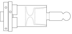
Cut the body and head of the doll to shape. Start the parting-off cut. Sand this part. Complete the parting-off cut. Set this part aside
