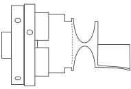
Cut below the seat of the chair to make a thin stem. Start the parting cut below the base of the chair. Sand all surfaces. Complete the parting off and hand sand the bottom of the chair.
