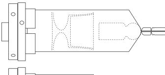
Mount the wood in a chuck. Turn it round. Cut down to 8mm diameter at the tailstock end. The longer pieces are the doll's arm - note the notch that is the wrist. The shorter pieces are shoes. Sand before parting off using the tip of a skew chisel. Set these pieces aside.
